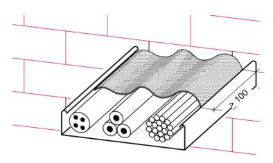
Step 2: Wrap the cables/ cable bundles and cable trays with "ZZ 451"
